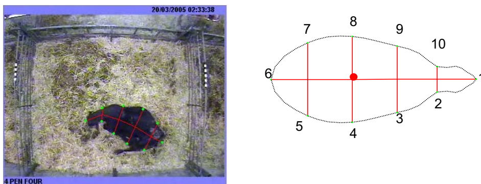
Figure 1. Screenshot of the image analysis output and the 2D model used. The model output consists of 10 points at consistent positions along the outline of the animal.
